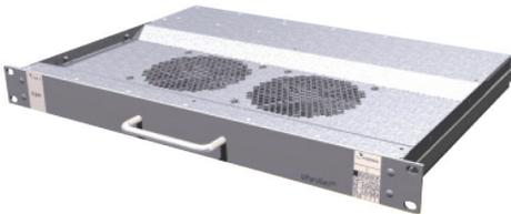
Depending on the ambient temperature, the fan speed is regulated linearly in a range between 50% and 100%. Besides advantages such as less noise generation as well as energy conservation, it also increases the life time (MTBF) of the fans. To make a diagnosis, the states "over- and under-
